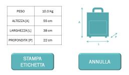
LOGISCAN Compact can be used simply as a measuring instrument: by inserting the baggage into the machine, the measurement system is immediately started, which provides the passenger with data on the weight and dimensions detected.
